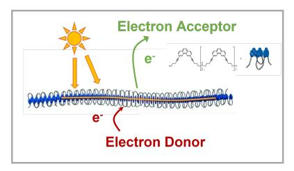
Photoinduced electronic transfers mediated by light-harvesting supramolecular phenanthrene polymer (in blue)
